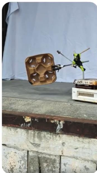
SAMPLE #2: (With 3.5% chitin nanocrystals dip coated)
